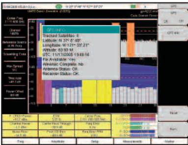
The MT8222A can easily enhance the frequency reference oscillator accuracy to make precise frequency error measurements.
